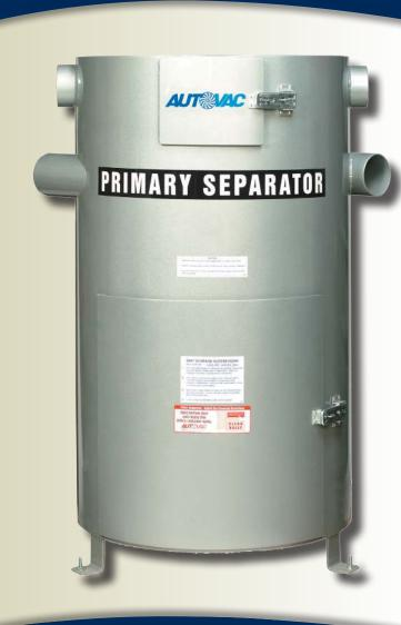
AutoVac's Primary Separator – your central vacuum system's first line of defense in filtration. "Dirty" air is pulled through vacuum hoses and piping, and then directly into the primary separator. Waste and debris pass around a precisely engineered baffle and then drop out of the air stream through centrifugal action. Debris drops into a waste container while air and any remaining particles move on to the filter separator (see Filter Separator page).
